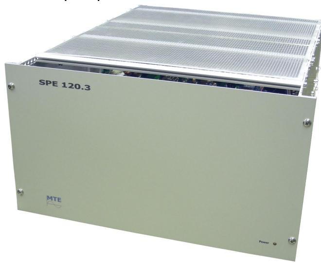
The SPE 120.3 is a three-phase computer controlled voltage and current source, designed for used in meter test systems and in the laboratory. It is in two performance steps with 300 VA and 600 VA output power available. The models are housed within a 19"-plug-in unit, 6 or 9 height modules, depending on output power.
